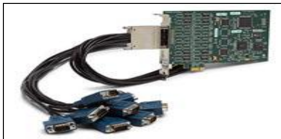
Figura 12. Interfaz RS232 de 8 Puertos, PCI Express.
