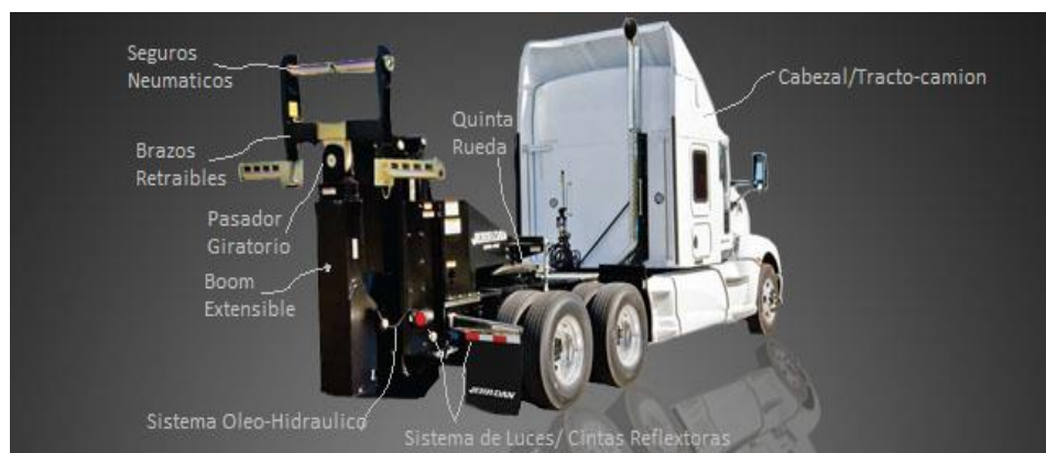
Figura 24 Partes del Sistema Under-Lift/Wheel-Lift. 25
