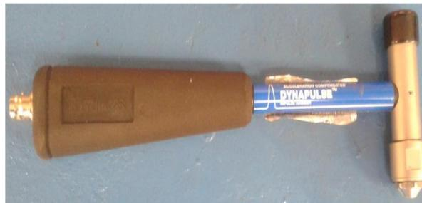
**Figura 2. 18:** DYTRAN modelo 5800B3, Dynapulse™ Impulse Hammer.
