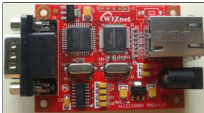
Figura 21. Conversor serial/Ethernet wiz110sr de WIZNET.
