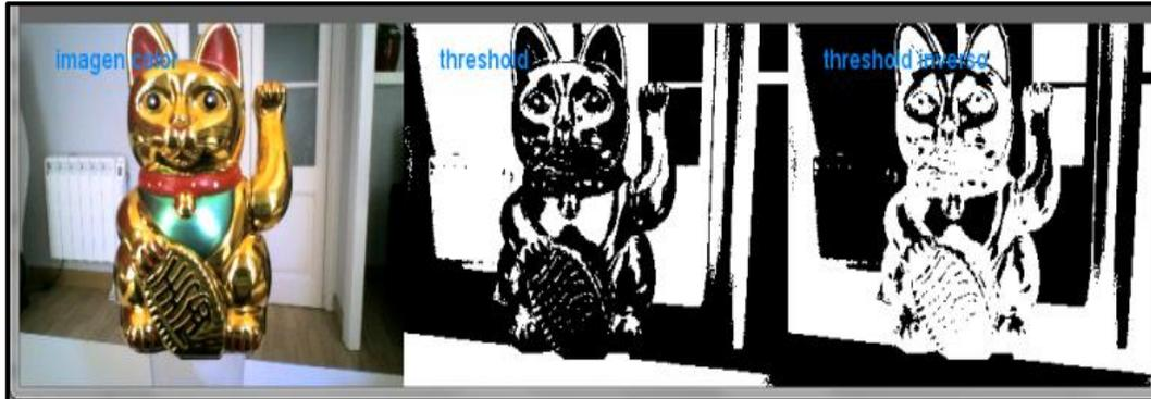
FIGURA N 6. EJEMPLO DEL USO DEL THRESHOLD
