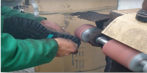
A close-up photograph showing a person's hands, wearing a green long-sleeved shirt, holding a shoe's sole against a rotating red sanding drum. The sole is being shaped and smoothed. The background shows a workshop environment with cardboard boxes and other equipment. |
