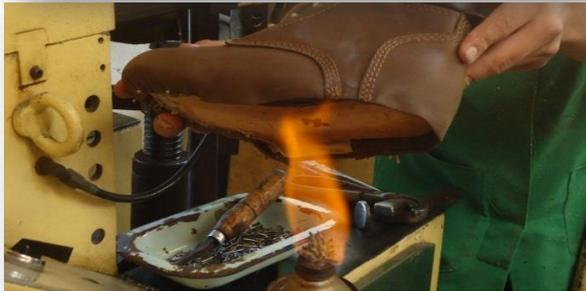
A close-up photograph showing a person's hands holding a brown leather shoe. A blowtorch is being used to heat the sole of the shoe, with a bright orange flame visible. The person is wearing a green shirt.           |
