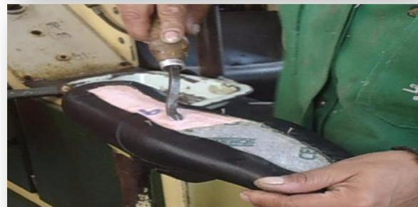
A close-up photograph showing a person's hands using a tool with a curved, pointed end to remove staples from a shoe insole. The insole is pink and black. The person is wearing a green shirt.                        |
