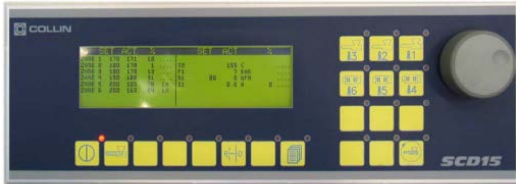
Figura 1.20: Panel de Control
