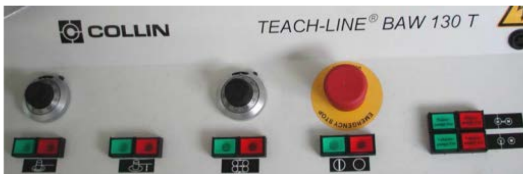
Figura 1.49: Panel de Control "BAW 130 T" + "WR 650 T"
