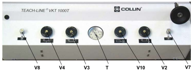
Figura 1.45: Tablero de Control "VKT 1000 T"
