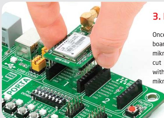
Once you have soldered the headers your board is ready to be placed into desired mikroBUS™ socket. Make sure to align the cut in the lower-right part of the board with the markings on the silkscreen at the mikroBUS™ socket. If all of pins are aligned correctly, push the board all the way into the socket.
