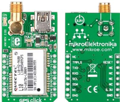
GPS Click - L10 is an accessory board in **mikroBus™** form factor. It's a compact solution for adding GPS functionality to your device. It features **Quectel® L10**, high performance MTK positioning engine. GPS Click - L10 communicates with target board through UART or I<sup>2</sup>C interface. Data can be acquired using PC application through USB connection. Board features connector compatible with active and passive antennas. It can operate on 3.3V power supply only.
