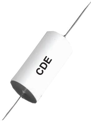
**Type 942C** round, axial film capacitors utilize a hybrid section design of polypropylene film, metal foils and metallized polypropylene dielectric to achieve both high peak current as well as superior rms current ratings. This series is ideal for high pulse operation and high peak current circuits.
