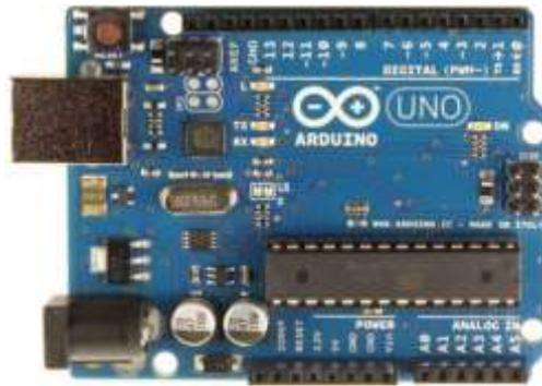
**Figura 2.1:** Tarjeta Arduino “Uno”
