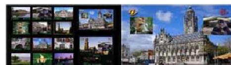
Way 3: HDMI 1 Multiscreen1- 8 smaller windows for inputs 1-8 with embedded audio level indication (group1, channel 1) + 2 bigger windows for Preview and Program. Embedded audio level indication for Program (group1, channel 1)
