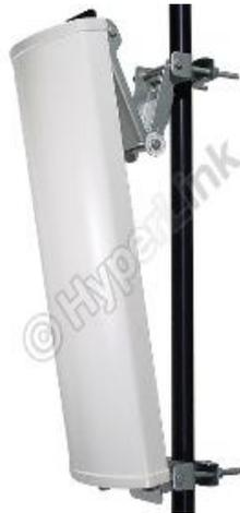
**Figura 3.16** Antena sectorial panel 2.4 ghz 14dBi
