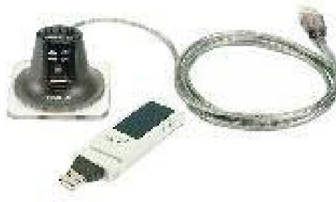
**Figura 3.10** Tarjeta inalámbrica 3COM OfficeConnect USB 108 Mbps 11g
