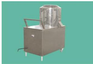
This equipment can mix floury, grainy material; it's the first step of food processing. It use “**工**” shape mixing method, drive by a electromotor, mainly using for mixing raw material, water and additives. Raw material mixed fast and evenly.
