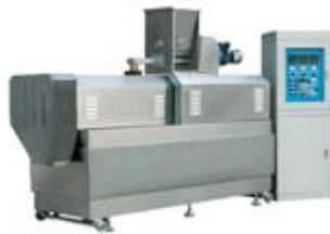
The twin screw extruder consists of material feeding system, extruding system, roll cutting system, heating system, driving system lubricating system and controlling system.
