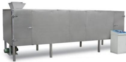
The three layers dryer is to and fro structure, it contains transmission electrical motor, stainless steel carrying belt, infrared heating pipes and supporting frame. As snacks go through the drier, they will be dried quickly in a clean condition. In the corn flakes production line, this drier can dry materials quickly after presser step.
