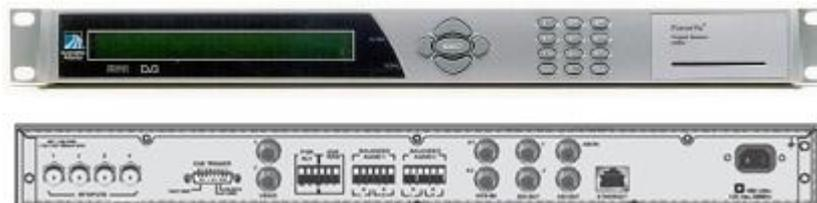
Figura 8 Receptor satelital, PowerVu Modelo D9850 4RF
