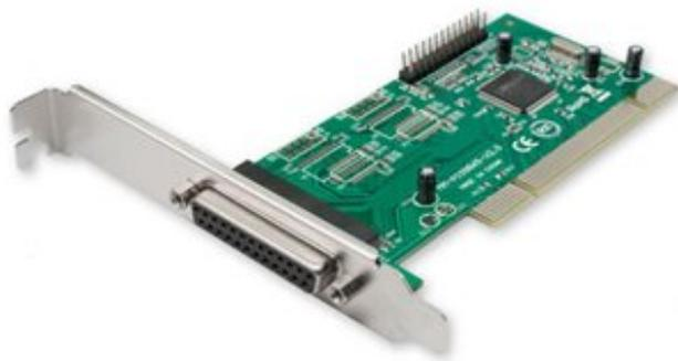
**Figura 1.3:** Tarjeta Bus PCI [1].
