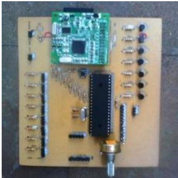
Figura 4.16. PCB principal terminada de Circuito Principal
