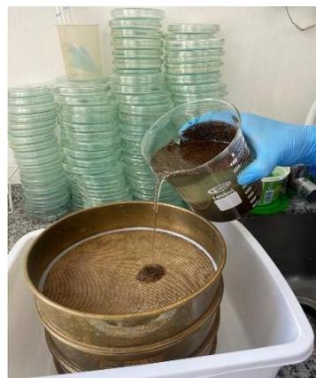
A person in blue gloves is pouring a liquid suspension from a glass beaker through a stack of sieves into a white bucket.                                                 |
