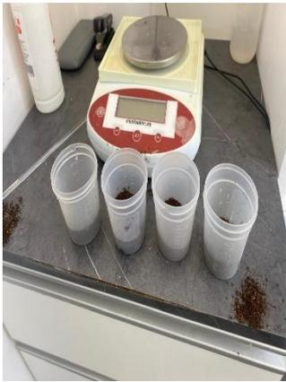
A digital scale is used to weigh soil samples into four white plastic cups. The scale is on a lab bench with other equipment.                   |
