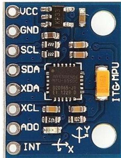
Figura 7. Sensor MPU6050 [22]
