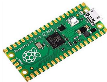
Figura 10. Raspberry Pi Pico [101].
