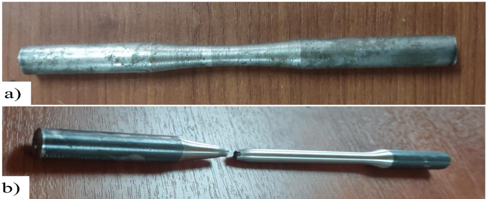
Figure 2 Specimen a) machined, b) after tensile test
