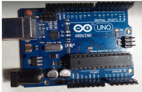
Nota. Arduino uno (Arduino.cl, s.f).
