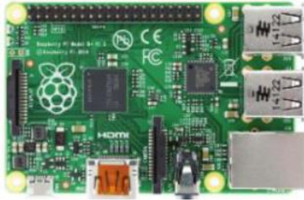
Figuras 5 Raspberry Pi 1 modelo B+
