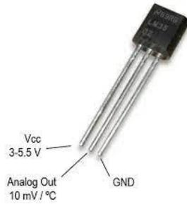
*Nota. Transistor de Sensor LM-35 (Texas Instruments., 2019)*
