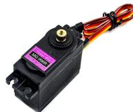
Figura 8. Servomotor MG996R [26]
