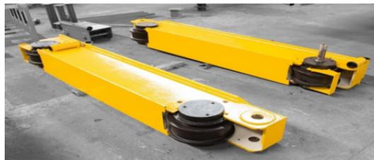
Figura 13: Unión viga- Testeros [26].
