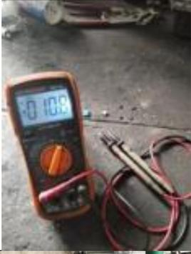
A digital multimeter with a red and black casing, showing a reading on its LCD screen, with test leads connected.    |  |
