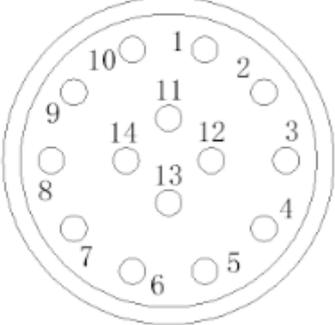
**Figure 5:** The connecting diagram of J1 and J2
