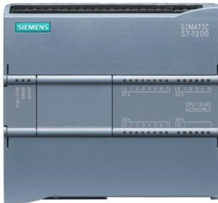
Figura 3. PLC S7 1200 AC/DC/RLY [4]
