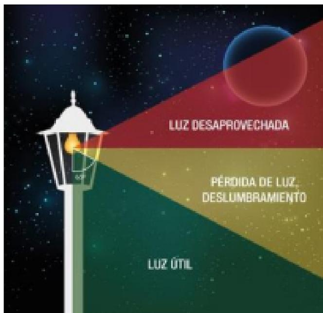
Figura 10: Deslumbramiento
