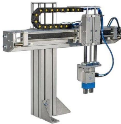
Figura 9. Pick & Place Unit de FESTO [20].
