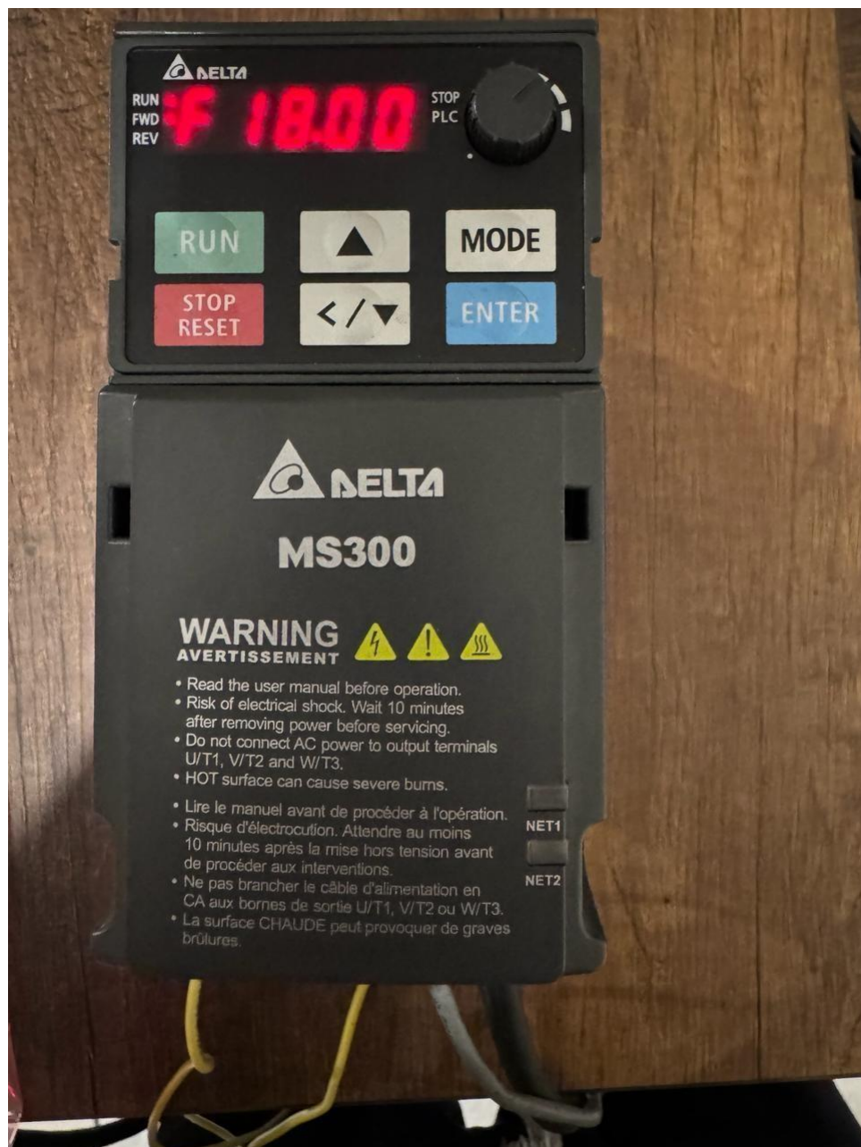
Figura 3.31: VFD giro horario
