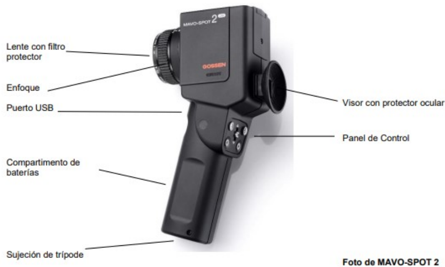
Figura 3.2: Luminancímetro GOSEN MAVO-SPOT 2 [4].
