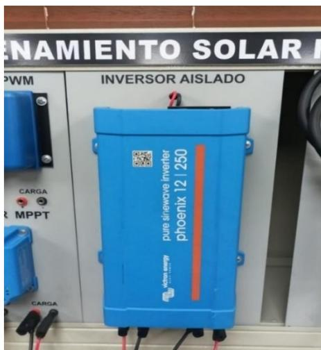
Figura 16 Inversor aislado, [6]
