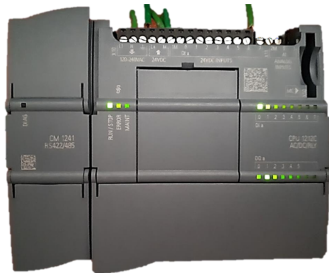
Figura 11. PLC SIMATIC S7-1200 CPU 1212.
