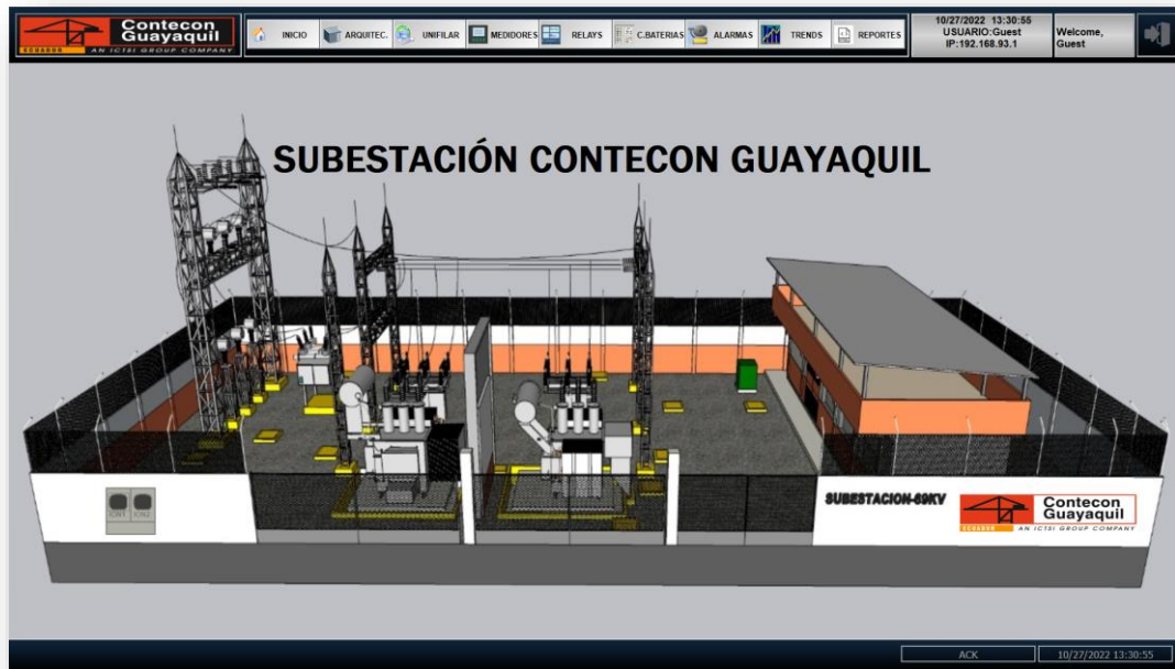
Figura 29: Pantalla Principal SCADA
