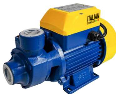
Figura 10: Bomba periférica 1/2 hp – 30l/min – 110v/220v
