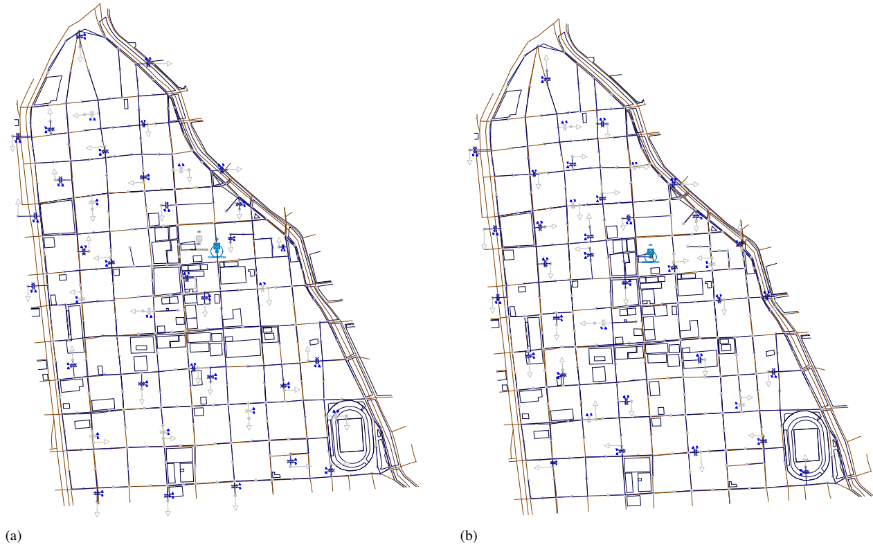
Figure 7: a) K-Means reconnected by feeder failure 3. (b) K-Medoids reconnected by feeder failure 2.
