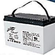
DC (Deep Cycle) series batteries provide superior high integrity and reliability. It is specially designed for frequent cyclic charge and discharge. By using strong grids, thick plate and specially active material are designed for repeated deep-discharge applications. The DC series batteries offer 30% more cyclic life than the standby series. It is suitable for solar and wind renewable energy storage, mobility and medical equipment, V, telecom, broadband and cable TV, UPS systems etc.
