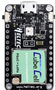
Figura 2.1: Cube Cell HTCC-AB01.
