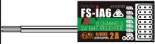
A small, rectangular 2.4GHz receiver module, model FS-IA6. It has a green PCB and a black plastic housing. The text on the module includes "FS-IA6", "6 CHANNELS", "2.4 GHz RECEIVER", and "CLASS 2A".                               |
