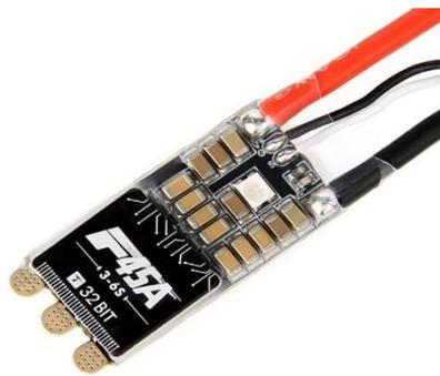
**Figura 35.** Vista frontal ESC T-Motor F45A. [27]
