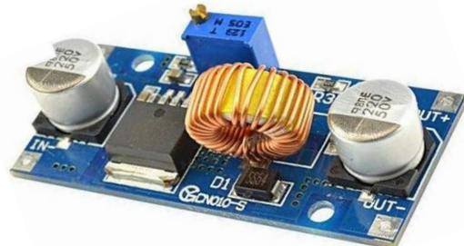
Figura 15. DollaTek XL4015 5A DC-DC (Electronico Caldas, 2019)
