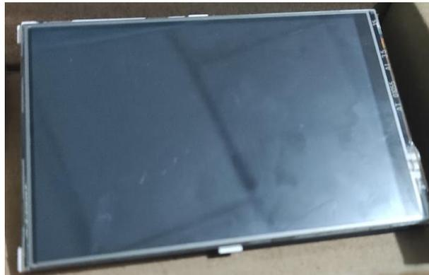
*Figura 9.* WS 3.5inch RPi LCD.
