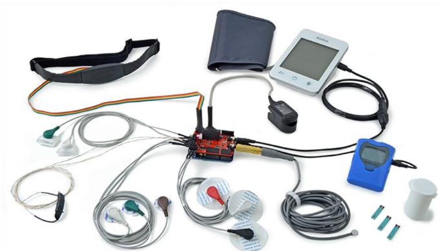
**Figura 7:** E-health sensor shield (SoloElectronicos, 2017)
