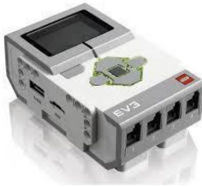
**Figura 5: Bloque de control Mindstorms**
