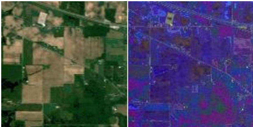
(a) RGB color remote sensing image of the Indian Pines. (b) RGB color Multispectral remote sensing image of the Indian Pines after applying MNF preprocessing.
