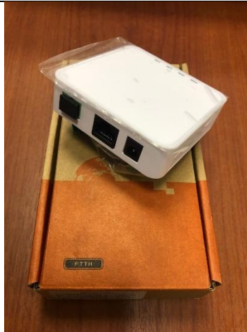
Figura 103 ONT FTTH 1 puerto ETHERNET, 1 puerto PON
