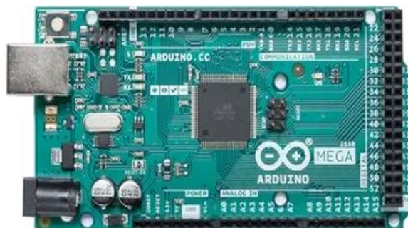
Figura 2.11 Arduino Mega 2560 Autor: (Electronics, s.f.)
