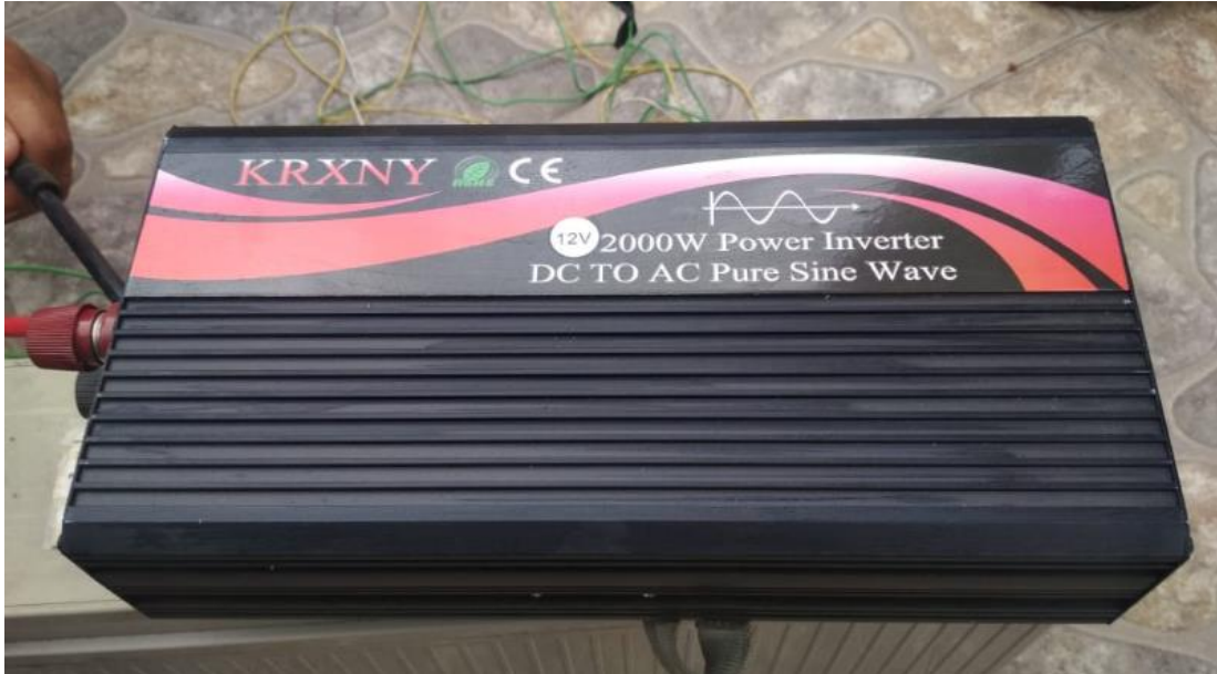
Figura 27. Inversor KRXNY 12VDC/ 120 V RMS Sinusoidal pura (AMAZON, 2020)
