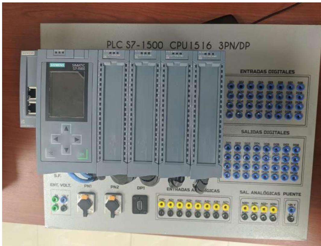
Figura 35. Panel PLC S7-1500 CPU1516 3DP/DP.
