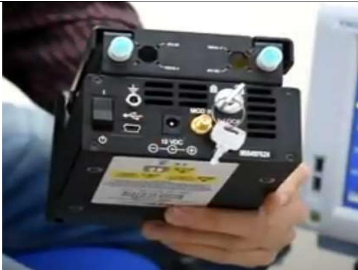
Figura 47. Compact Laser Diode Controller CLD1015
