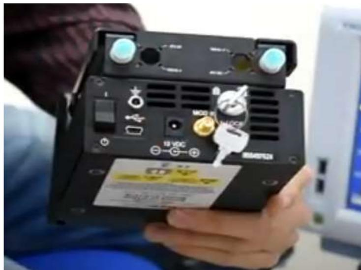
Figura 4.3. Compact Laser Diode Controller CLD1015
