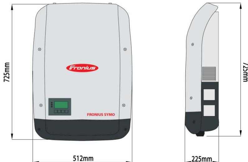
Figura 2-32 Inversor Fronius SYMO 20.0-3-M.
